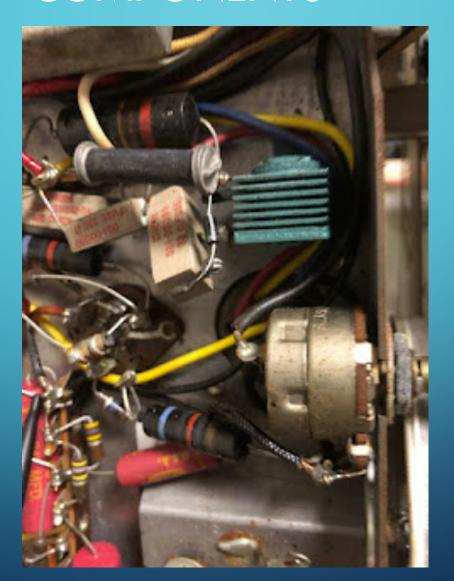
Selenium diode (green device) replaced with 1N4007 diode - the large black component is a "glowbar".
